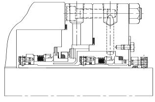
A dual seal arrangement with a diverter (option). Type 609HTC inner seal with a Type 609HTC outer seal. Typically used with API Plan 54.
