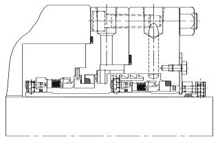
A dual seal with a Type 609HTC inner seal and 609HTC outer seal. Typically used with API Plan 52 or 53A.
